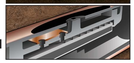
XFS emitters are protected from root intrusion by Rain Bird's patent-pending Copper Shield Technology resulting in a system that does not require maintenance or replacement of chemicals to prevent root intrusion. The copper color outside ensures the copper chip is inside.
